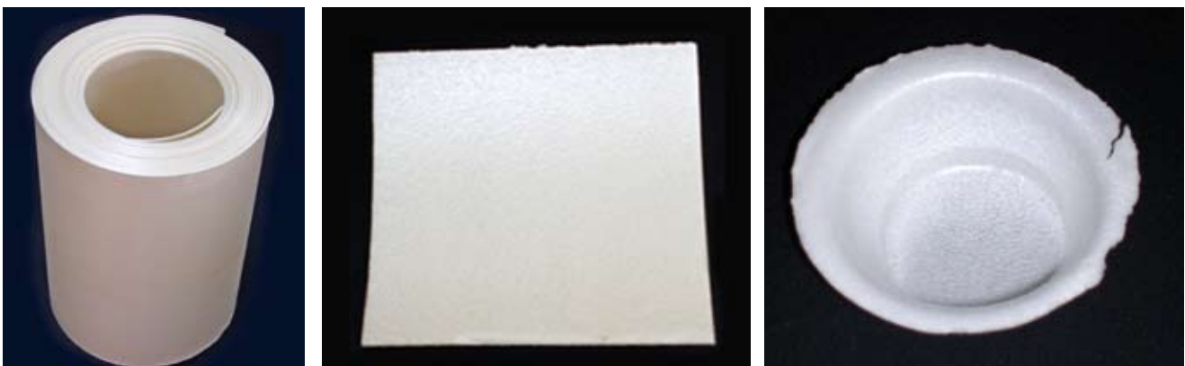
Fig. 1: Cellulose Acetate based foam sheets (right and centre) and thermoformed cup (left).
